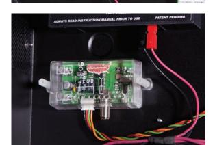
Install Entrapment Siren into the control box using the 2 nylon nuts provided as shown. Use a  $\frac{1}{4}$ " nut driver to secure. Connect the Siren power leads to the J4 Terminal as shown.
