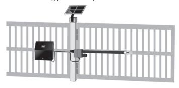
When deciding where to mount the control box remember the actuator cable is 8 feet in length. If possible, mount the control box in a location that will allow the cable to be neatly routed. If it must be longer than the 8 feet, see Step 13b pg 22 Splicing Actuator Cable. Also avoid choosing a mounting location that is near sprinklers.
