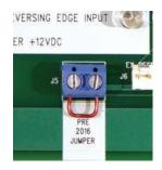
For this input to operate in pre-2016 mode you MUST turn on DS2 dipswitch 4.
