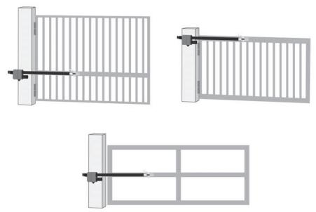
Installation of a horizontal brace may be necessary to prevent damage to vertical gate pickets.
