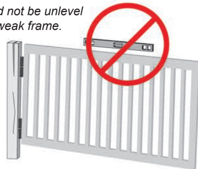
Gate should not be unlevel due to unlevel post.
