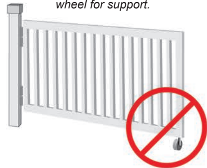
Gate should not require a wheel for support.
